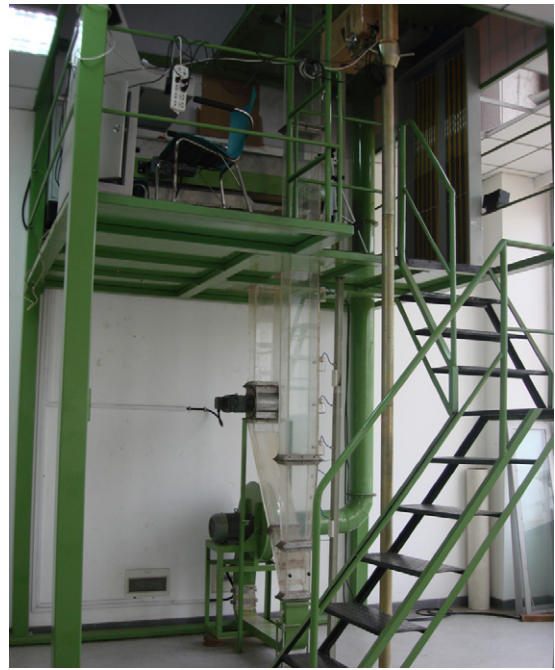
Fig. 9. Present rectangular fluidized bed.
